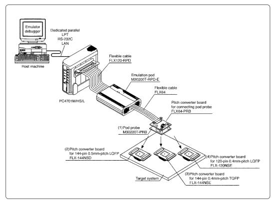
Figure 2.1 System configuration
